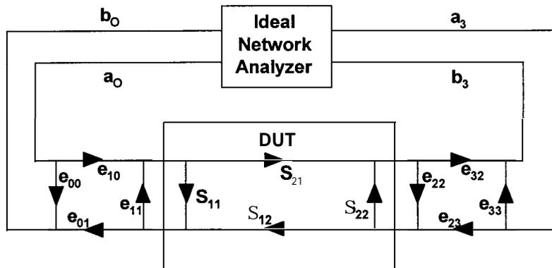
Figure 18. Signal flow graph of the switch corrected two-port VNA eight-term error model. Since S-parameters are ratios, only seven unknowns must be determined to complete the calibration.
