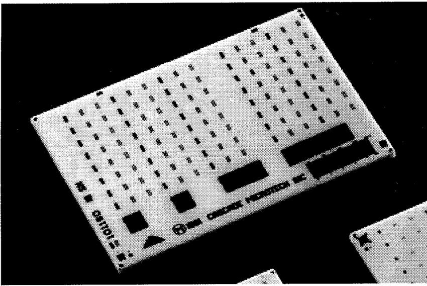
Figure 10. The LRM Impedance Standard Substrate (ISS) has multiple repeated patterns of Short-Load-Thru Standards and alignment marks for setting proper probe separation. A set of transmission lines are also provided for TRL Calibration.
