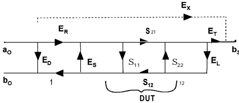
Figure 17. Signal flow graph of the full two-port VNA error model without switch corrections. The forward stimulation case is shown, a similar error model is used for reverse stimulation.
