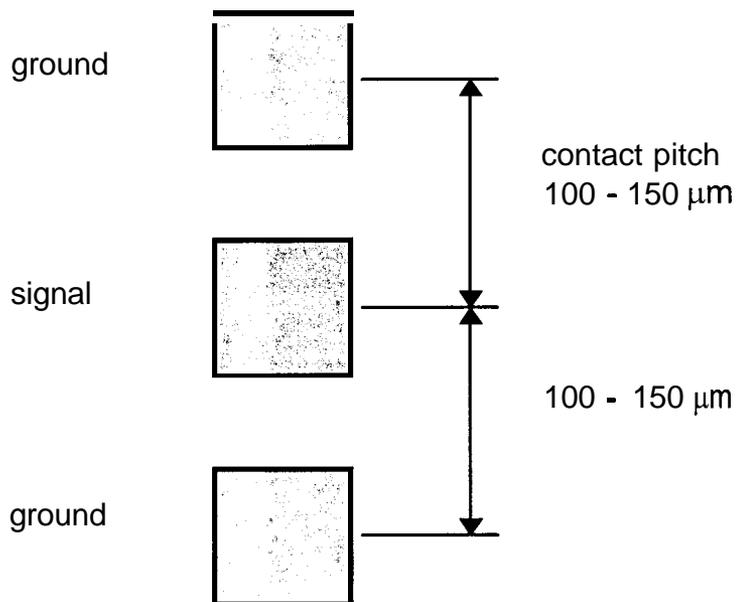
Figure 6. Recommended microwave pad pattern for each measurement port.
