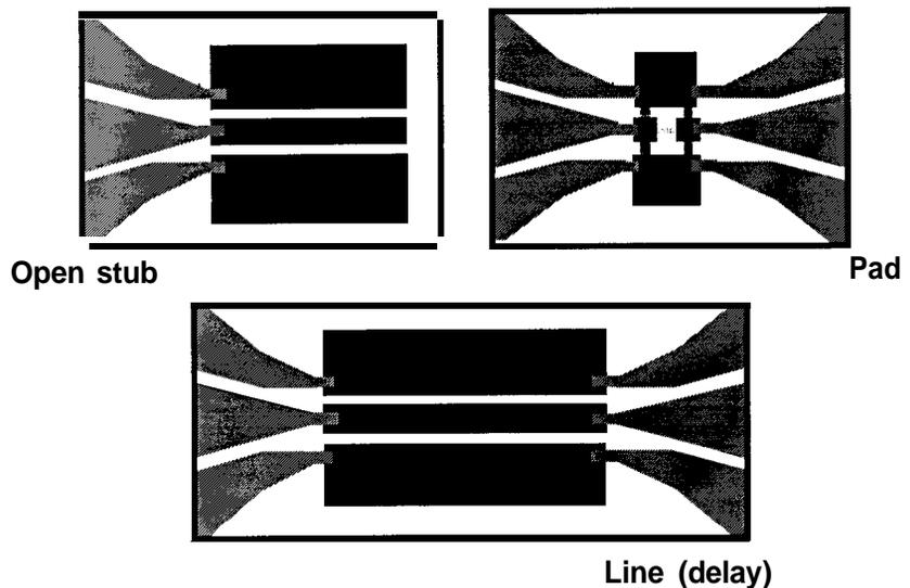
Figure 21. Typical on-wafer verification elements. In many cases measurement of such structures will catch the most common errors and problems.
