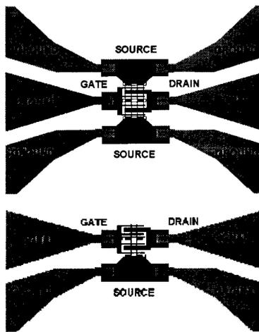
Figure 11. Microwave probe contact patterns. The Ground-Signal-Ground (GSG) pattern has higher performance than the Ground-Signal (GS/SG) configuration.
