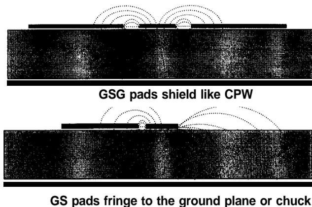
Figure 22. GS pads fringe to the ground plane or chuck.
