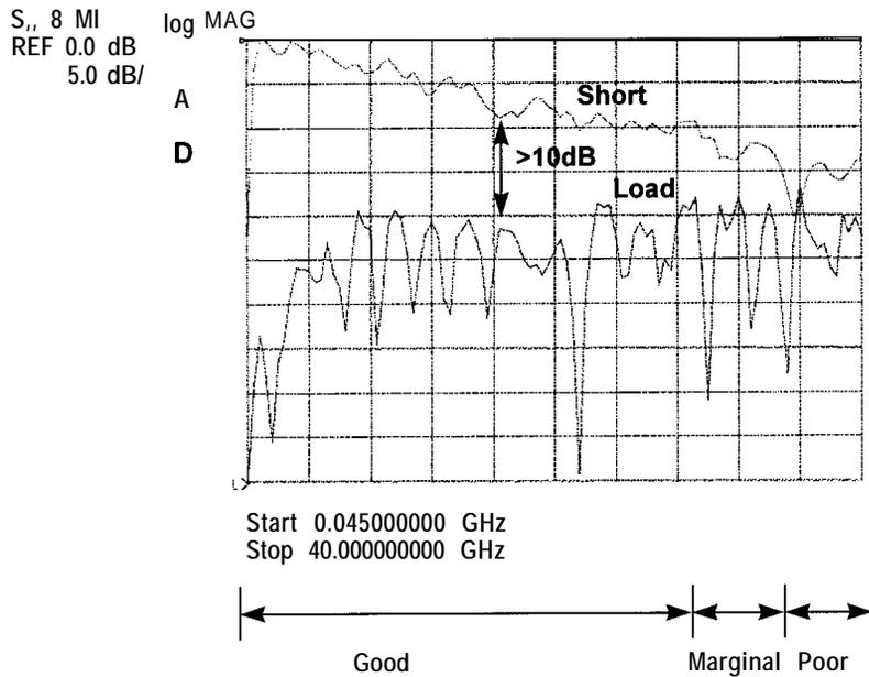
Figure 20. The relative magnitudes of uncorrected measurements of a short and a load provide a good check on proper system function.
