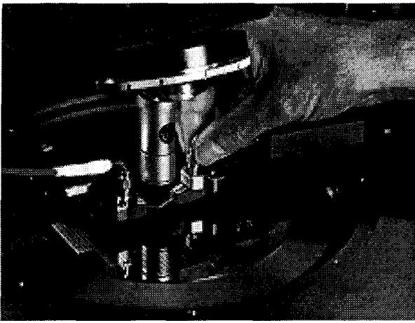
Figure 3. Close-up of microwave probes and cables on positioners providing probe planarity adjustment and cable restraints.
