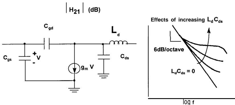
Figure 14. Inductance,  $L_d$ , due to layout inductance can resonate with device output capacitance and distort the measured frequency response.
