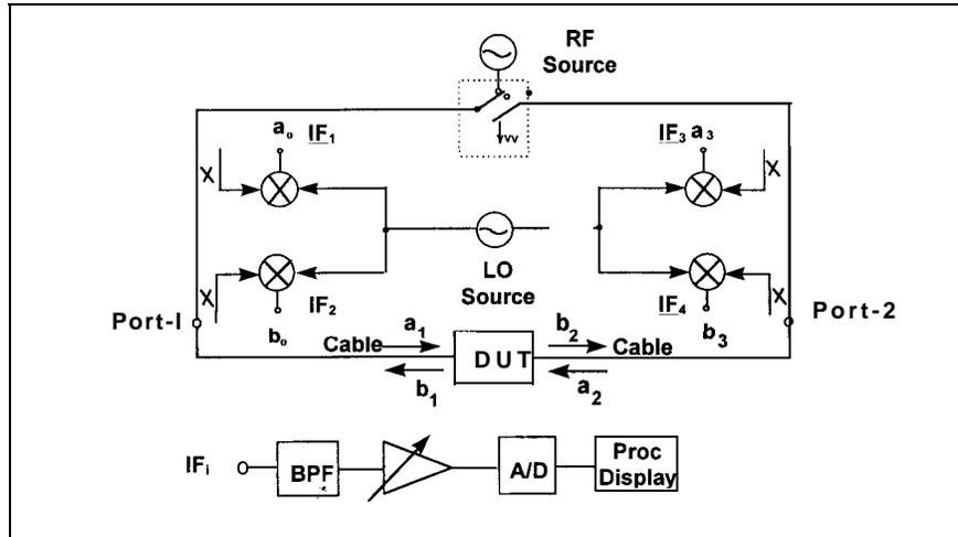
Figure 1. Main hardware blocks in a Vector Network Analyzer (VNA).
