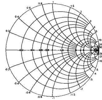
Figure 5. The Smith Chart is a polar graph of reflection coefficient with grid lines showing normalized impedance values.
