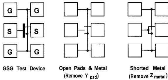
Figure 12. Pad Parasitic Removal structures.
