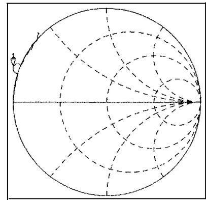
Figure 24. Calibrated measurement of short circuit standard before and after distressing a cable. A change has occurred in the cable electrical behavior resulting in a 20 GHz resonance.
