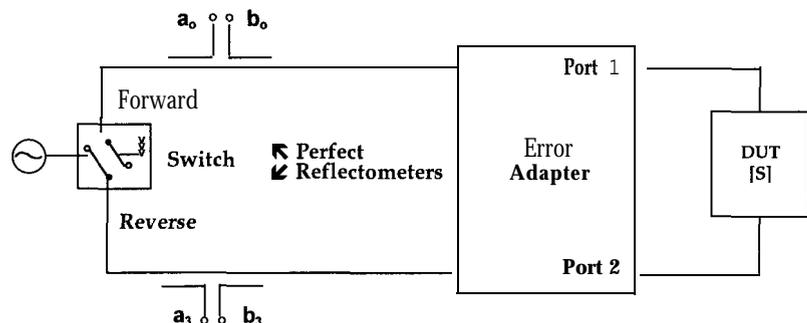
Figure 4. Error model for a typical network analyzer. All errors are modeled by an error adapter in front of an otherwise perfect system.
