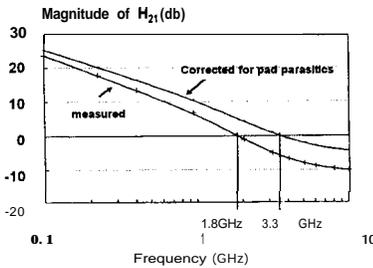
Figure 13. Apparent bandwidth improvement due to removal of pad parasitics.
