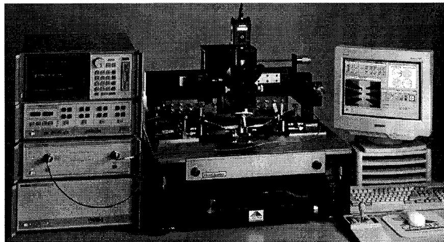
Figure 2. A typical RF device characterization setup is shown above. On the left is a vector network analyzer, in this case an Agilent 8510 system. Cables from the test set ports route over the probe station to a pair of microwave probes which are aligned through the microscope or camera system onto calibration substrates and test devices. The right side of this picture shows the PC that controls the prober and runs the calibration and measurement software.
