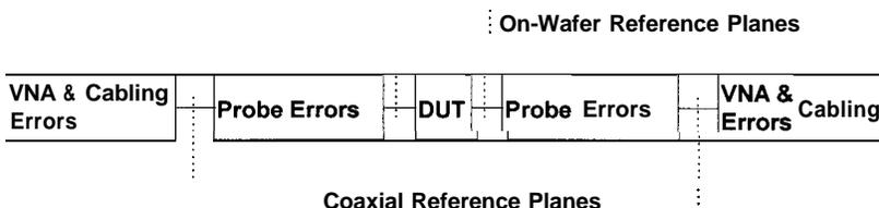
Figure 19. Error boxes for a two-tier calibration. A coaxial first tier is followed by an on-wafer second tier.
