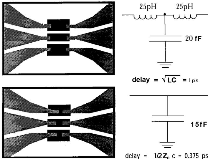
Figure 16. Improper probe placement will impact the electrical behavior of a measured standard. Use of alignment marks to set probe separation and reasonable care in placement will provide good results.
