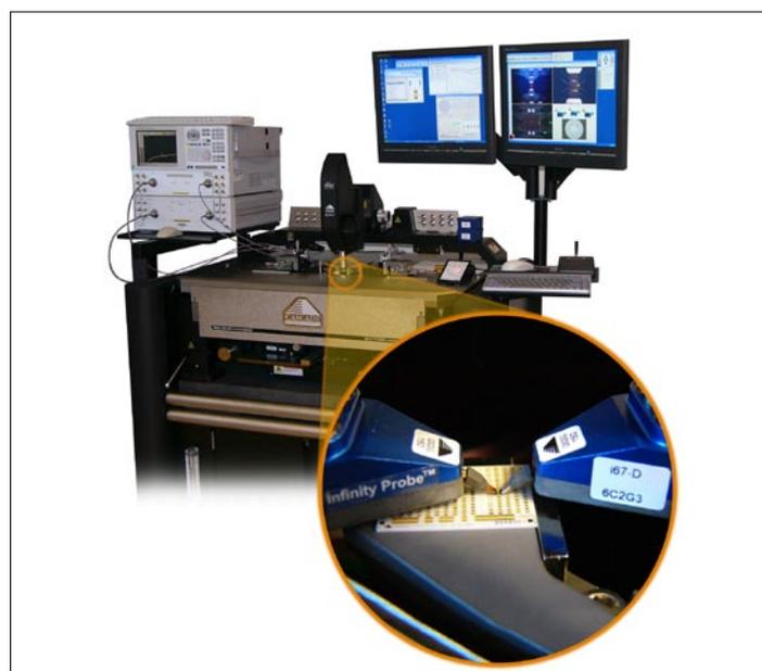
To get meaningful device data, the instrument must be calibrated so that the calibration reference plane is at the probe tip.
