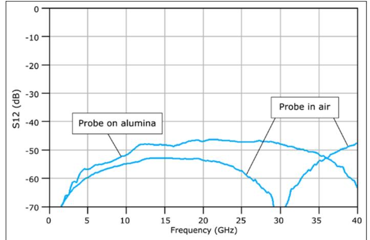
Cross-transmission line comparison of insertion loss of a hybrid calibration vs. a SOLT calibration. The SOLT calibration shows significant error; the hybrid calibration is clean.
