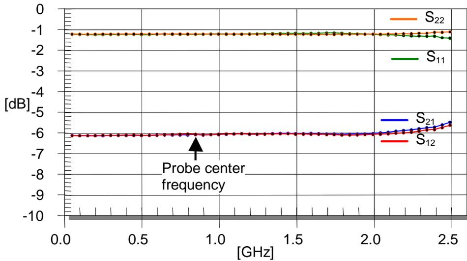
**Figure 4.** Measured normalized scattering parameters for a direct connection (1 ps Thru) between 50Ω port 1 and 3.5Ω port 2. The calibration succeeded over a frequency range much wider than the impedance matching probe bandwidth (10% centered at 0.85 GHz). The theoretically predicted normalized scattering parameters for this direct connection would be  $S_{11}=S_{22}= -1.22$  dB,  $S_{12}=S_{21}= -6.12$  dB.
