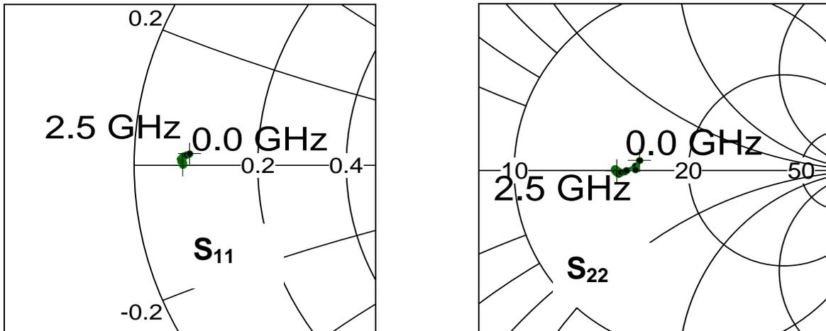
**Figure 5.** Expanded Smith Chart views of the measured normalized scattering parameters for the direct connection (1 ps Thru) between 50Ω port 1 and 3.5Ω port 2. The  $S_{11}=0.07$  value on the port 1 50 ohm normalized Smith Chart corresponds to measurement of the 3.5 ohm port 2 load. Similarly the  $S_{22} \sim 14.5$  on the port 2 3.5 ohm normalized Smith Chart corresponds to measurement of the 50 ohm port 1 impedance.
